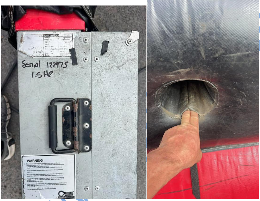
All 12 pole rests are worn out, 2 inch hole in each position needs repair
